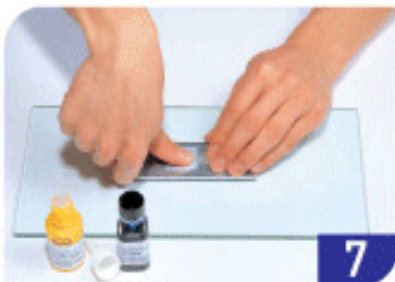
7 Pressing the strain gage
