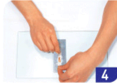
4 Aligning the strain gage
